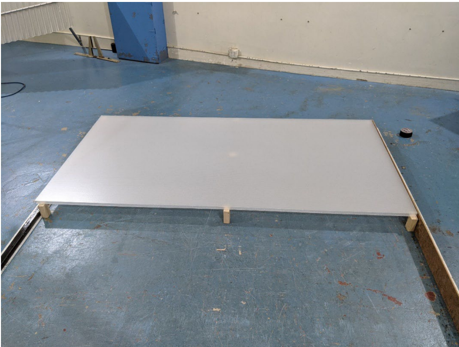
Figure 4 – Specimen partially installed over spacers
