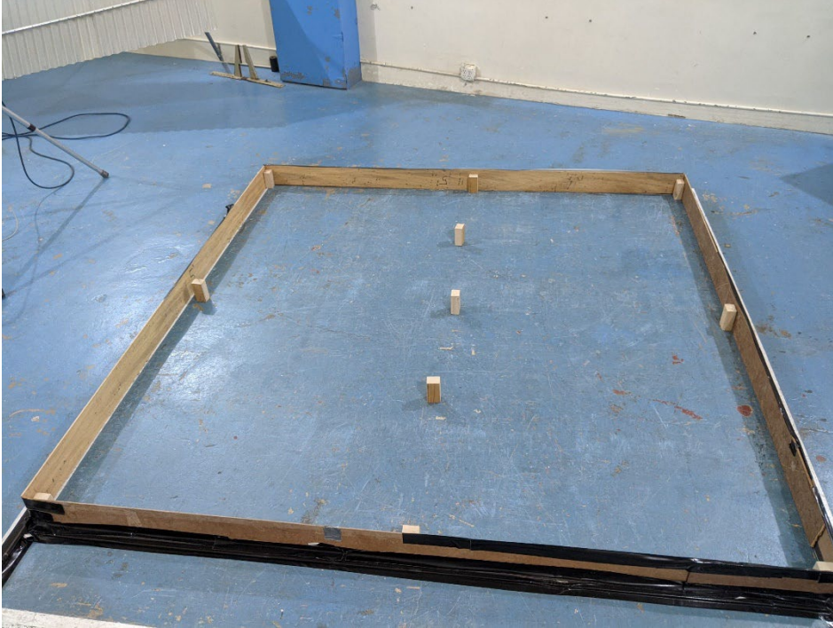
Figure 3 – Wood spacers in test chamber
