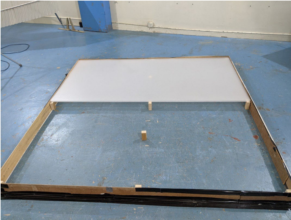
Figure 4 – Specimen partially installed over spacers
