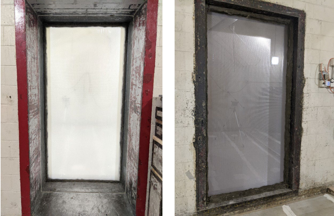
Figure 1 – Specimen mounted in test aperture, as viewed from source room (left) and receive room (right)
